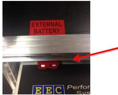
ANDERSON CONNECTOR FOR EXTERNAL BATTERY
